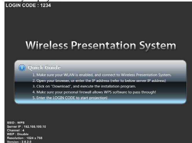
From the projector's screen, note the 4-digit Log-in Code, SSID and Server IP address. You will need this information to install the player software.
